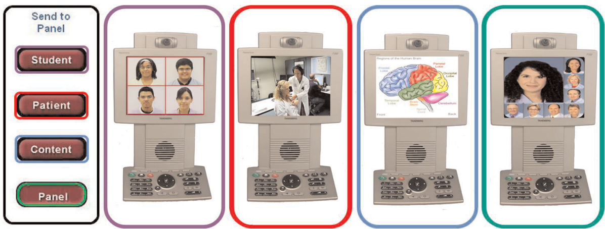
FIGURE 6. T-Health Amphitheater's Crestron display options, as would be viewed on the remote Tandberg T-150 video conference units by off-site faculty members (compare with Fig. 1). A representation of the T-Health Amphitheater Crestron touch-activated control screen is shown on the left. In this example, the classroom facilitator has selected "send to panel" and has four options (left to right): 1) send video/audio images of student e-Stacks to the expert panel members; 2) send the video/audio stream of the telemedicine clinic to the expert panel members supplied with T-150s; 3) send other content to the panel members, such as the brain mapping diagram shown on the T-150 video screen; or 4) send the eight-member expert panel members the video of the panel in which they are participants (right). Choice of the distribution option for the outgoing video content from the T-Health Amphitheater is managed by the facilitator at the amphitheater.
