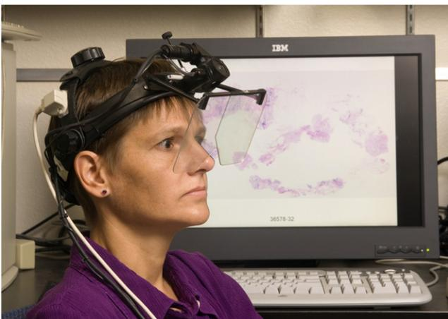
**Fig. 1** Eye position being recorded using an Eye-Tracker SU4000. An author (E.A.K.) is demonstrating the wearing of the eye tracker apparatus.
